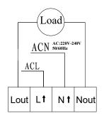
Fig.3 Wiring Diagram
